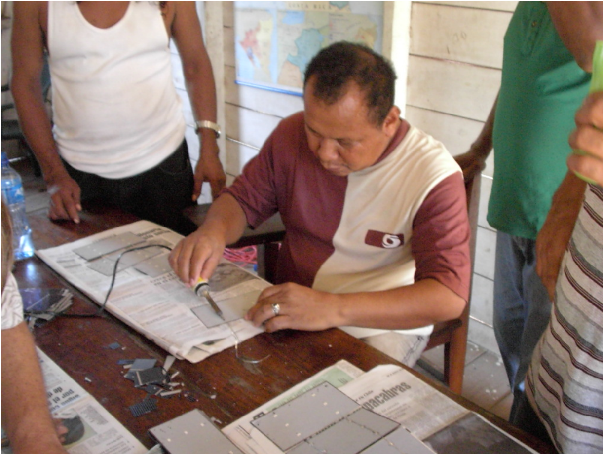
Photo 1 shows one of the Miskito Indians learning how to solder together the Evergreen Solar cells. 36 of these will be strung together to make a 60 watt PV module.
