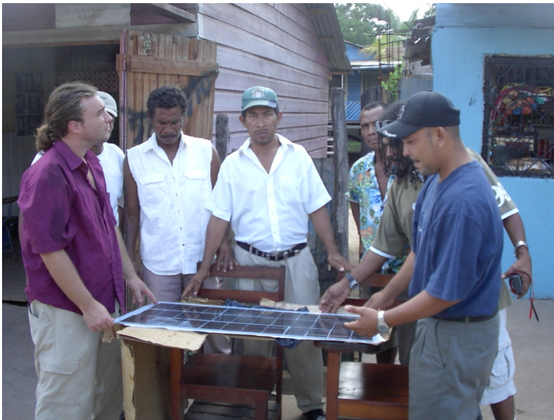
Photo 3. Testing the finished 60 watt PV modules the next day. Cody, on the left, is waiting for the sun to come out from behind a cloud to get a good reading.
