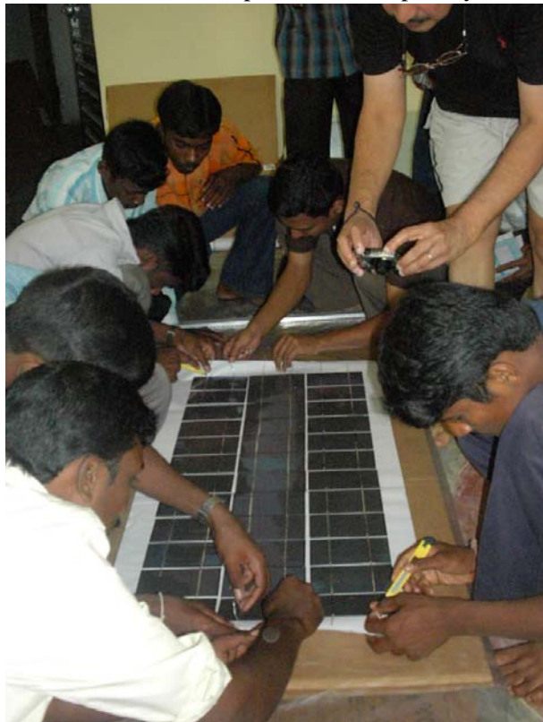
Photo 5, Making a 60 watt PV module
